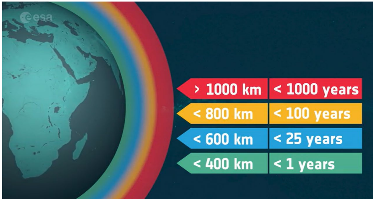
Figure 5: LEO de-orbit times (Credit: ESA)
